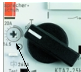
Handle in the tripped position
