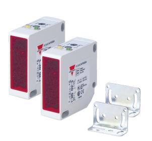
PC Series Photoelectric Sensor, Through-Beam, receiver and emitter, plastic housing, 12-240 V DC / 24-240 V AC supply, NO+NC output, 20m sensing range, IP67 rating, mounting bracket included
