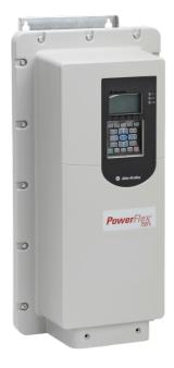
PowerFlex 753 AC Drive, 400 V AC, 3 PH, 15.4 A, 7.5 kW ND, 5.5 kW HD, Wall Mount - IP54, NEMA/UL Type 12, No Brake Resistor, Blank (No HIM)
